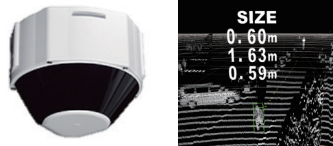
Fig. 5 Left: 3D LiDAR. Right: captured 3D LiDAR image presented on 3D viewer.
